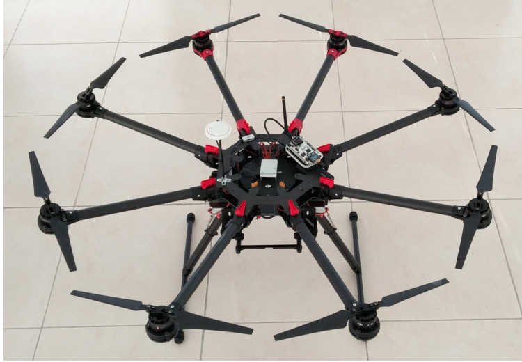
FIGURE B.13: DJI S1000 aircraft equipped with an IoT platform for the evaluation of various IoT protocols
