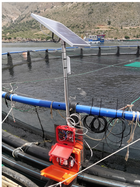
(A) Overwater System w/ Solar Panel
