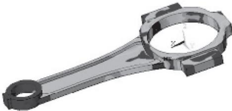
Figure 14 Model of a connecting rod using ANSYS finite-element software (Meshed model). [2]
