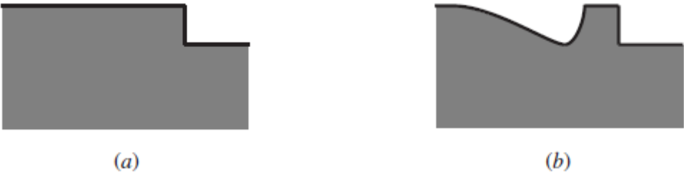
Figure 10 Guiding the lines of stress by means of notches that are not functionally essential is a useful method of reducing the detrimental effects of notches that cannot be avoided. These are termed relief notches. It is assumed here that the bearing surface of the step of (a) is needed functionally. Adding a notch as in (b) can reduce the hazardous effects of the corner of (a).[3]
