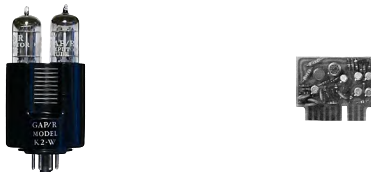
(A) GAP/R's model K2-W: A vacuum-tube op amp (1953).[3] (B) GAP/R's model P45: A solid-state, discrete op amp (1961).[4]
