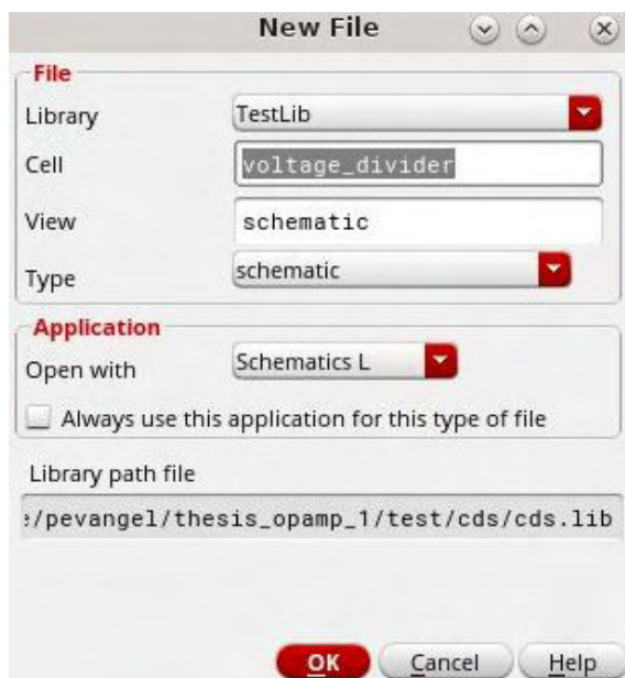
FIGURE 3.1: The "New File" window during the creation of a new cell.
