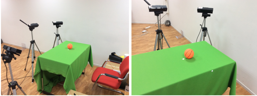
Figure 4-2: SOR3D capturing snapshots. The two markers on the tablecloth indicate the starting position of the object (at the middle of the table) and the hand (at the edge of the table).
