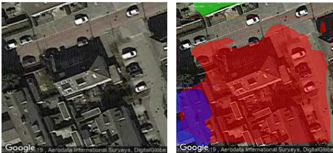
Figure 16a, 16b: A case of misclassification. The main causes of this issue are continuity in textures and colors along with the absence of vivid segregating objects.
