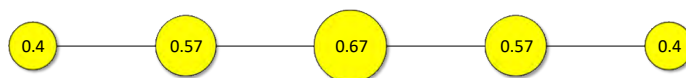
FIGURE 2.11. A closeness centrality example. Nodes towards the center of the graph are more prominent because, on the average, their geodesic distance from the other nodes in the graph is shorter.
