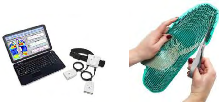
6: F-Scan Wireless System / Trimming of the sensors
