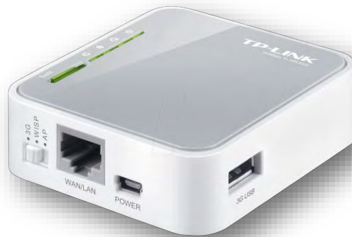
Figure 3 12 OpenWrt Router Tp-Link TL-MR3020
