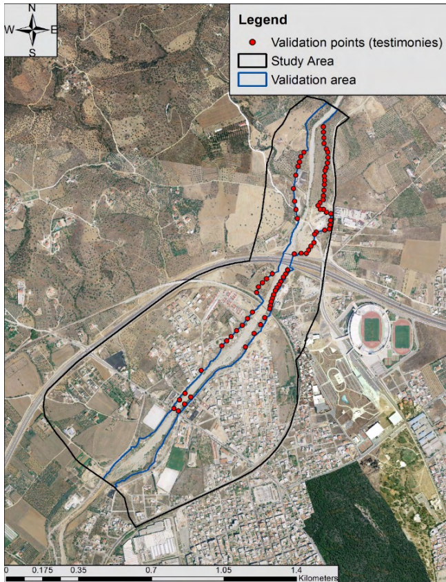
Figure 2.12. Flood routing stream reach reconstructed flood validation data.
