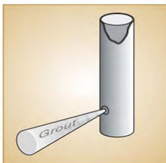
SINGLE JET Soil loosening and grout injection are performed by a jet of high pressure grout from nozzles at the bottom end of a drill rod.
