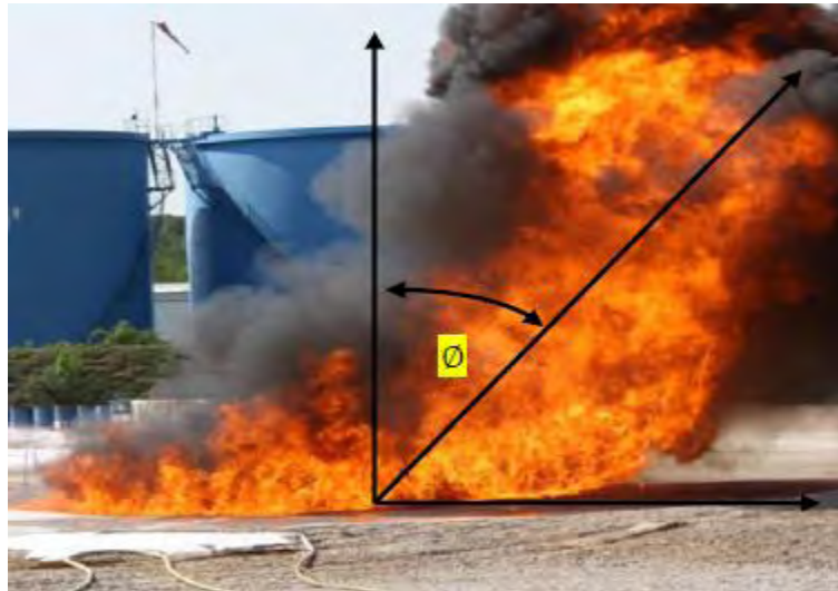
Figure 2-6 Flame tilt of gasoline fire (Mansour 2012)
