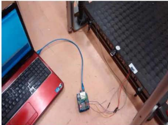
Figure 2.15. Laptop used as power source for the UNO board
