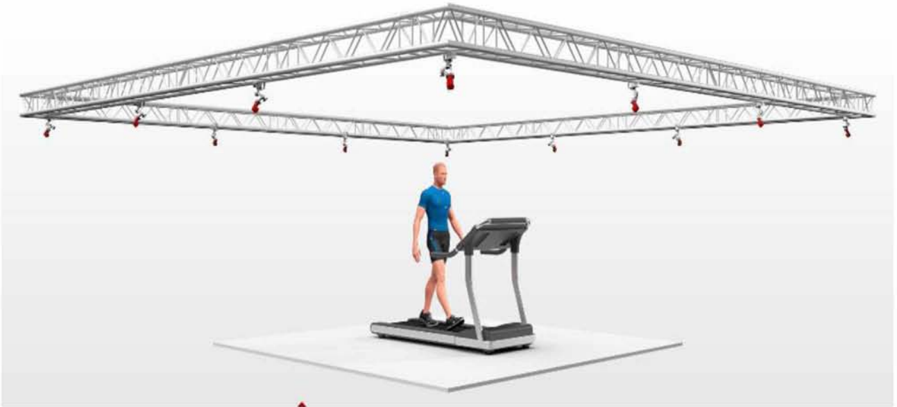
Figure 1.1. Camera set-up for Optitrack
