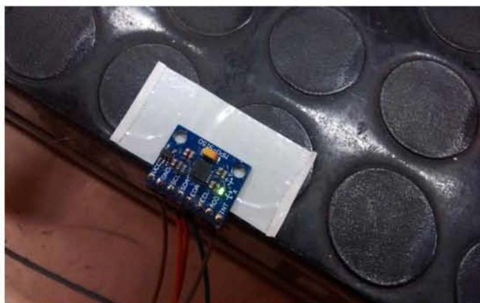
Figure 6.1. MPU-9150 taped on Posturomed platform
