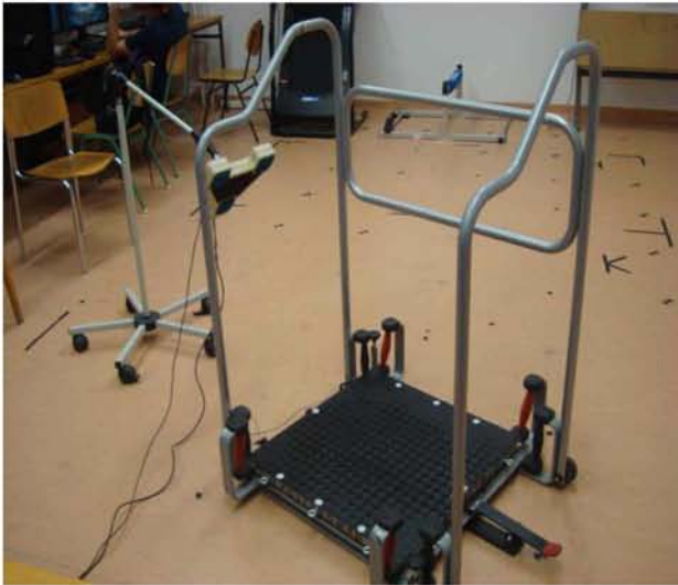
Figure 2.5 Zebris CMS10 placement relative to the Posturomed
