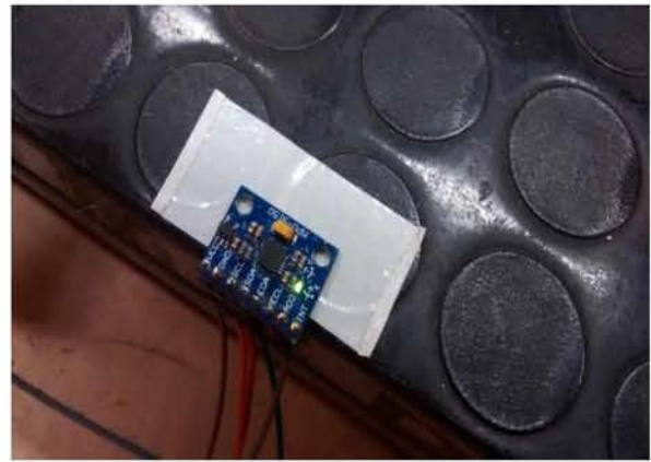
Figure 2.4. MPU-9150 taped on the Posturomed platform
