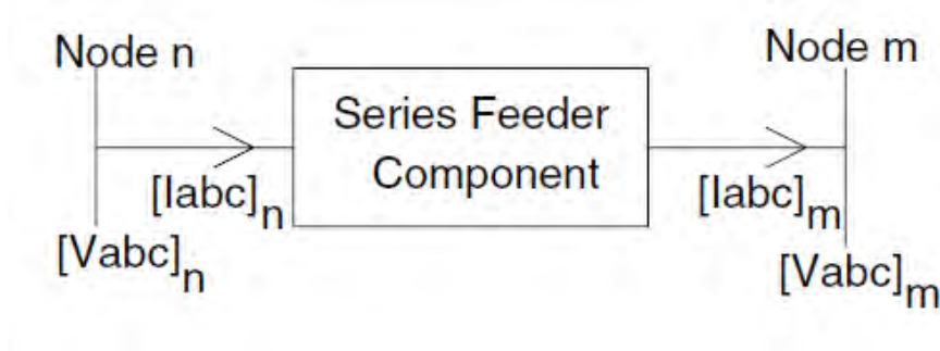
FIGURE 3.3: Three-phase line segment model
