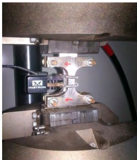
Figure 3.5 Strain controlled fatigue test setup with the use of anti-buckling device.
