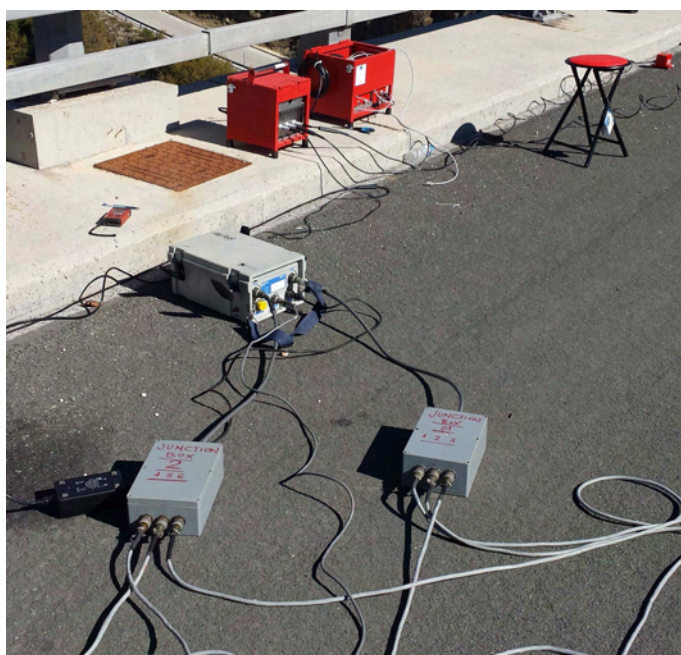
Figure 4.9: Junction box and unit including recorder, battery pack and GPS module
