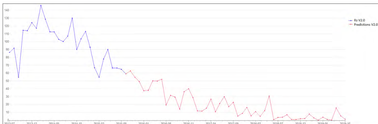
Figure 46 Extension of our monthly sunspot-number V2.0 predictions 50 steps ahead (September 2015 – October 2019). The blue curve corresponds to the actual sunspot-number V2.0 series; the red curve corresponds to our predictions using the V2.0 series as input data.
