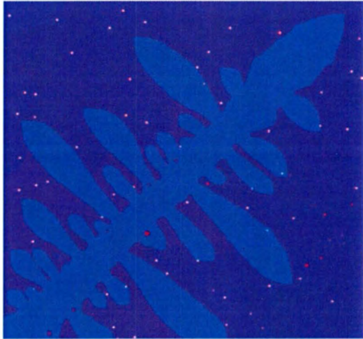
Figure 2.2.10: Solidification simulation in cast iron. The formation and the growth of tiny MnS particles in the liquid influence the subsequent formation of graphite [83].
