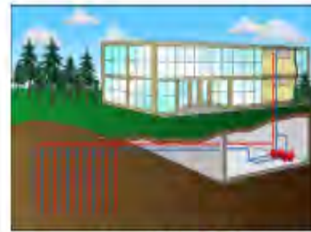
Ground-Coupled WSHP System
