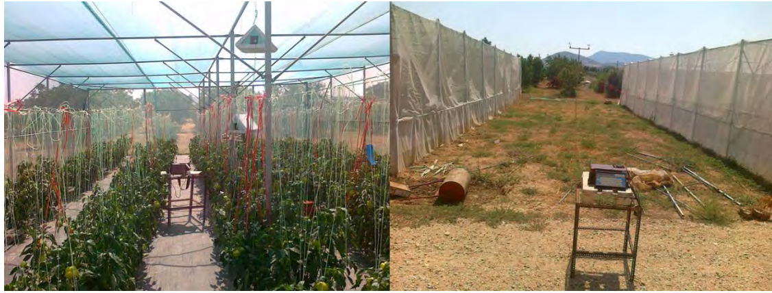
Figure 7. Photos during in situ measurements of light quality by means of a portable spectroradiometer LI-COR 1800. Left: measurement inside the screenhouse; Right: measurement at the open field.
