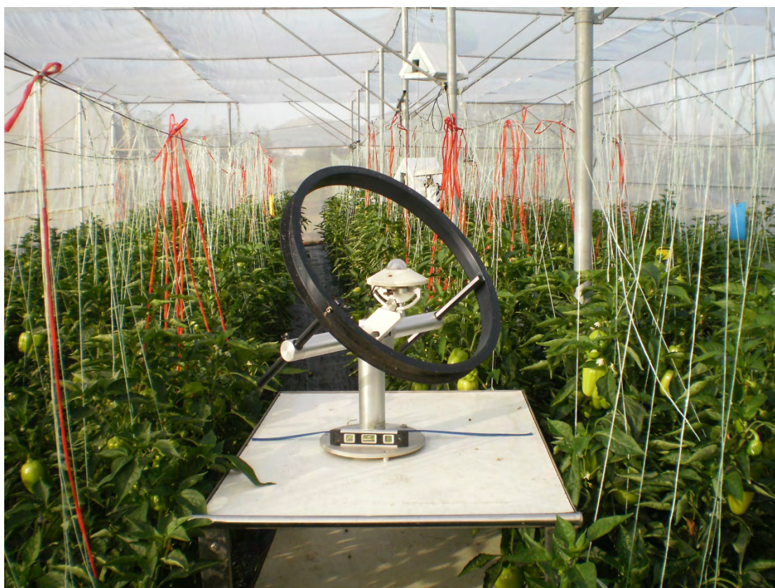
Figure 9. Shadow ring for diffuse radiation measurements.
