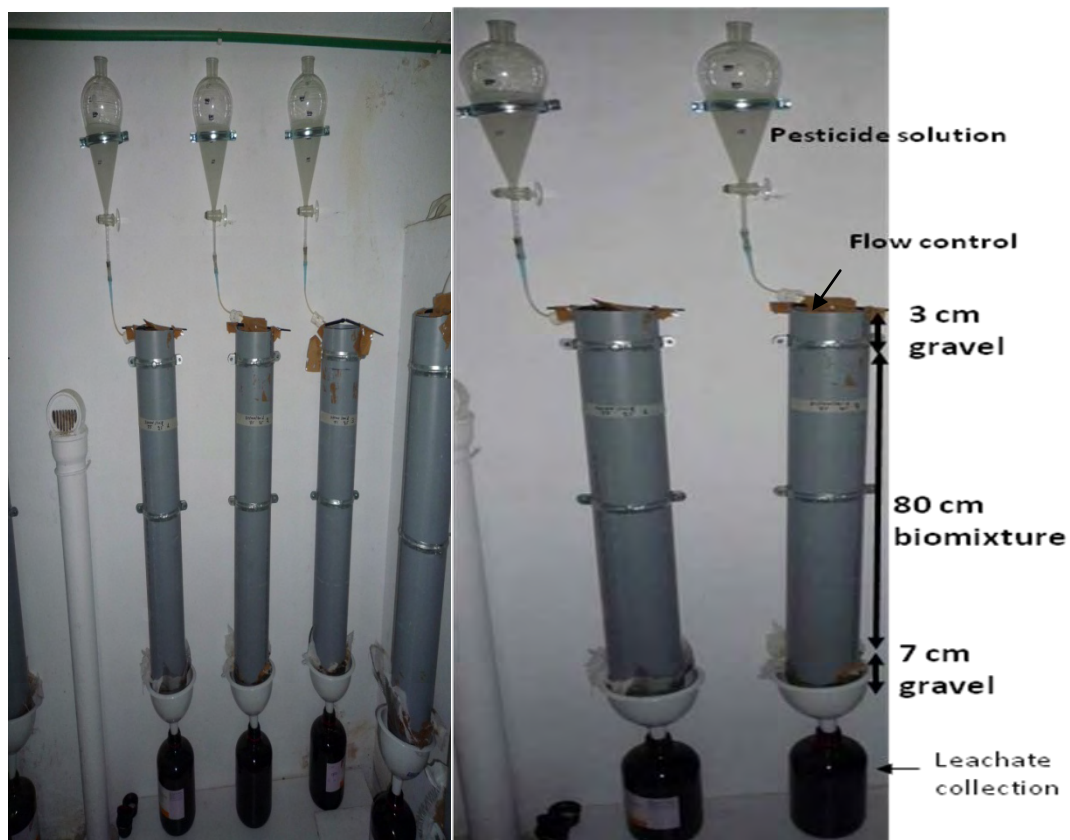
Photograph 3.1: The installation and the experimental set up of the leaching columns.
