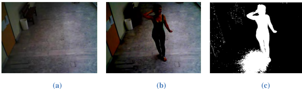
Figure 10. Two typical original frames acquired by one of the three projective cameras: a background image (a) and an image containing the object/human model (b). The corresponding segmented frame is shown in (c).
