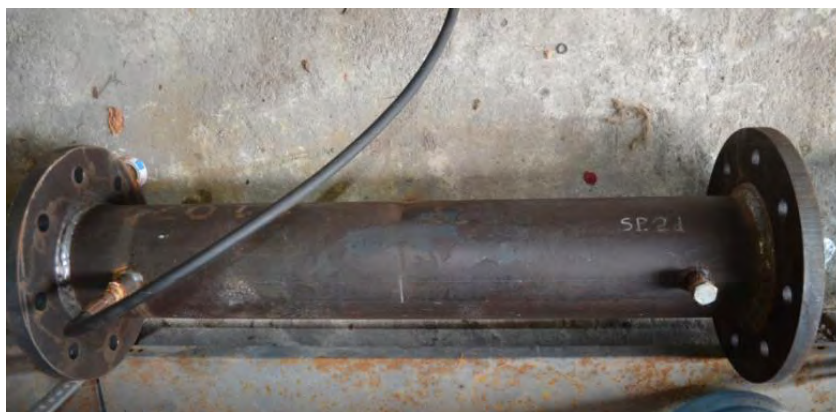
Figure 3-25: Pressure application on specimens \text{Ø}168.3/4.78 .
