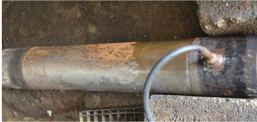
Figure 3-26: Pressure application on specimens \text{Ø}165/3 .
