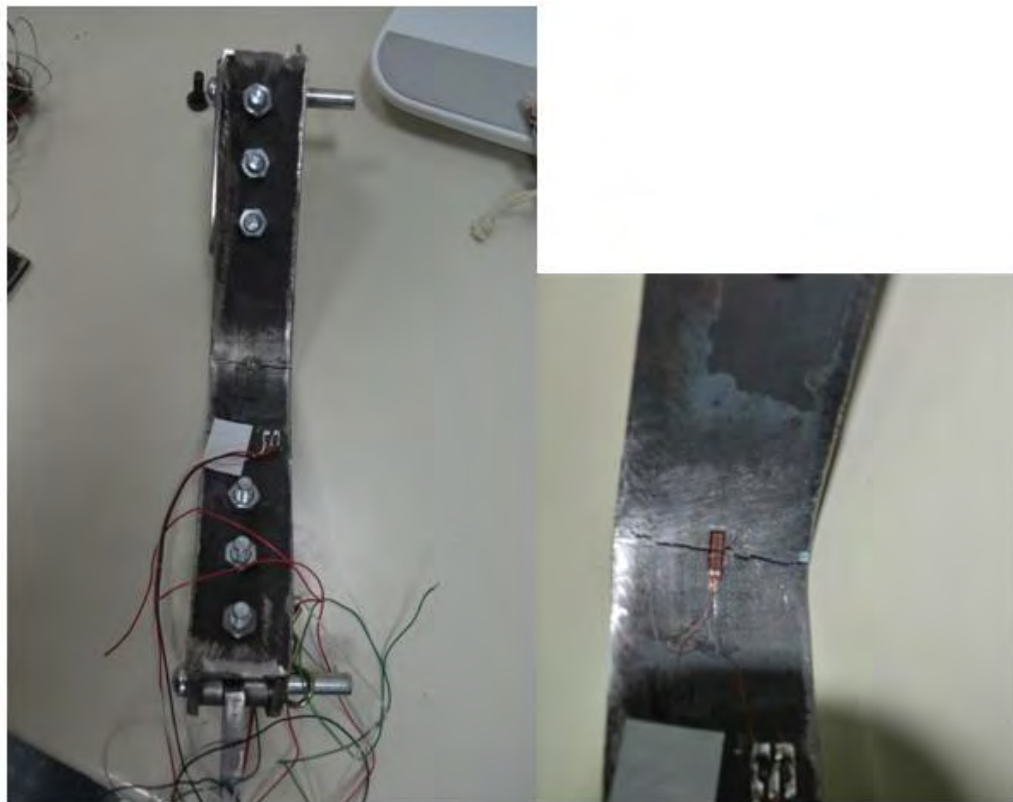
Figure 3-81: Crack development of specimen S21-View from the inner face of the strip. The crack propagated along the transverse direction.
