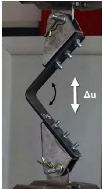
Figure 5-3: Loading and test configuration of strip specimens
