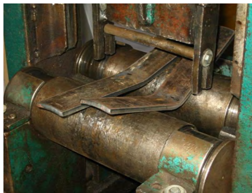
Figure 3-65: Monotonic 3-point bending loading
