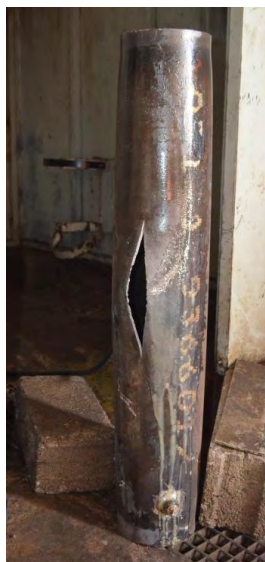
Figure 3-63: Rupture of perfect \text{Ø} 168.3/4.78 specimen
