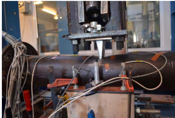
Figure 3-11: The stiffened wooden base
