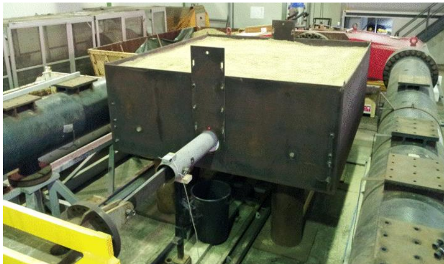
Figure 26. Setup of the pull-out tests before at the beginning of testing.
