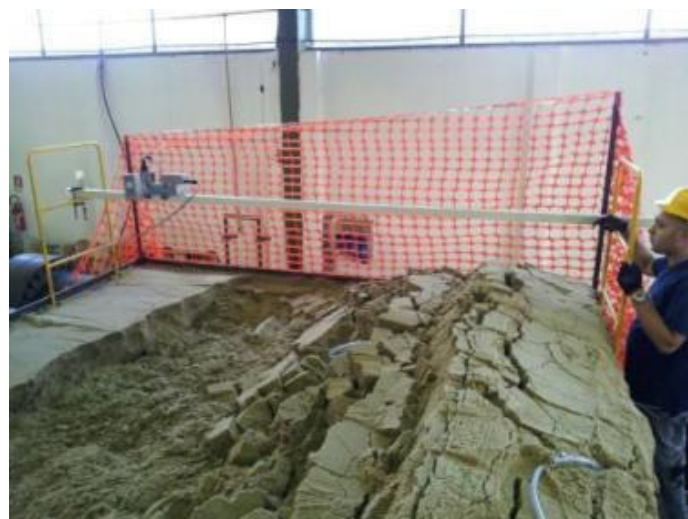
Figure 18. Deformed shape of the soil free surface at the end of the test.
