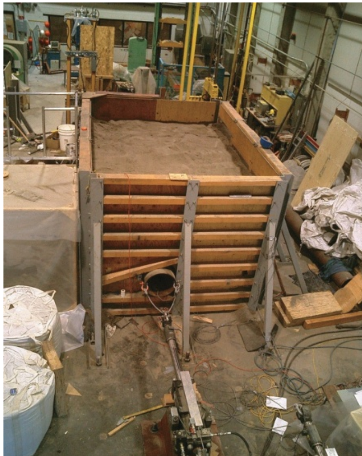
Figure 29. Experimental setup of axial test performed by Karimian (2006).
