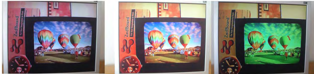
Figure 2.13: Different Options for Gamma (RGB)
