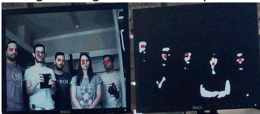
Figure 4.4: Face Detection and Tracking for 3-5 Faces
