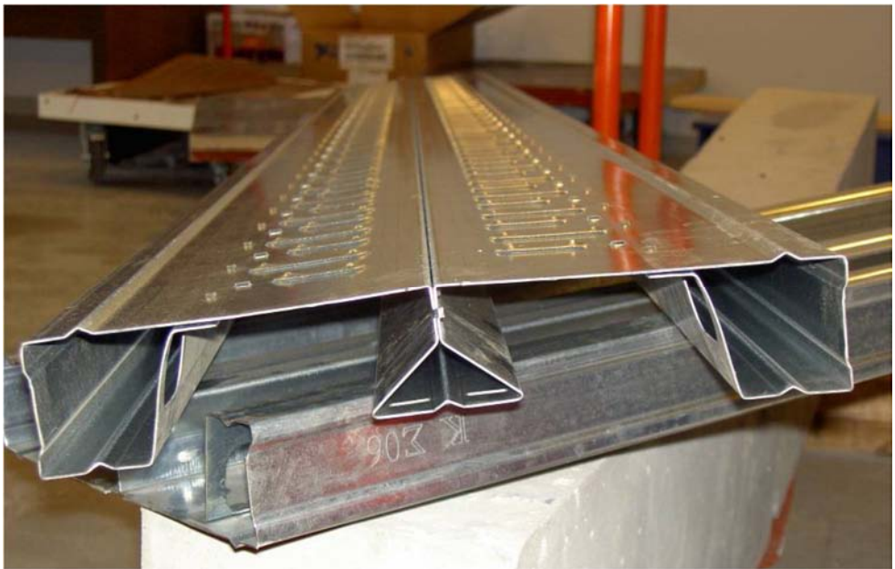
Fig. 2.1. The cross section of the thin walled cold formed steel beam (Tzaros and Mistakidis, 2008).
