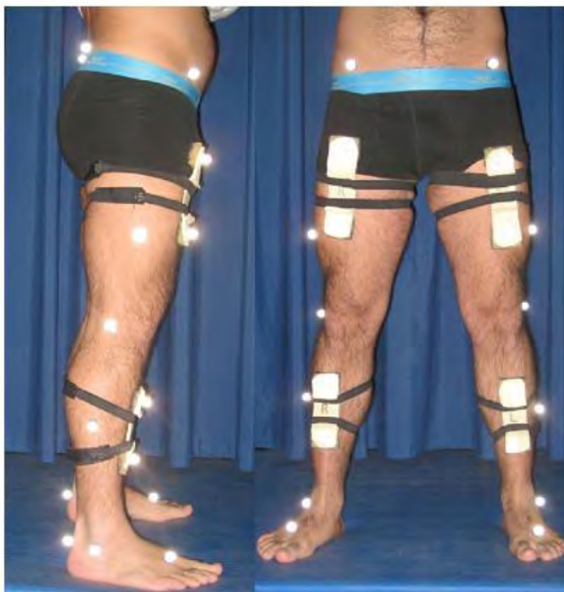
Figure 3. Position of 24 reflective markers. The model includes the well-known position of the 16 markers from Davis model with the addition of 2 markers positioned on a plate strapped tightly around the calves and thighs
