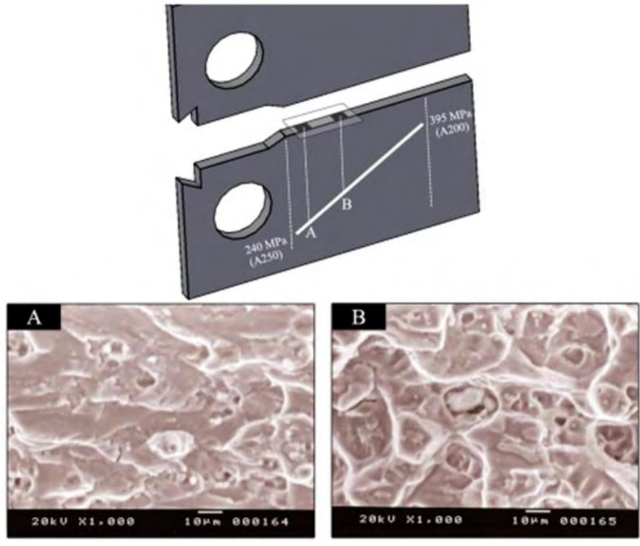
Figure 4.24 Fracture surface characteristics of specimen with positive strength gradient at \Delta K values a) \Delta K=11 \text{ MPam}^{1/2} b) \Delta K=20 \text{ MPam}^{1/2} .
