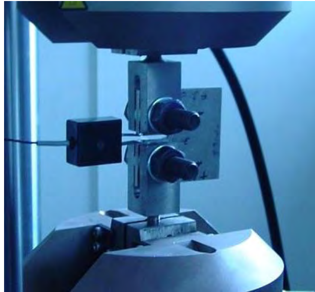
Figure 3.13 Fatigue crack growth test setup.
