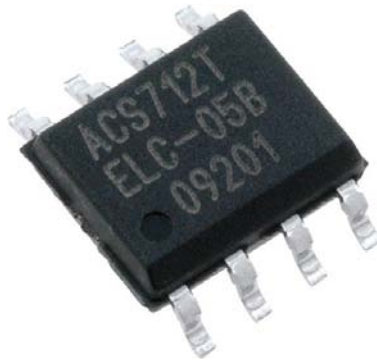
Figure 2 : ACS712 current sensor
