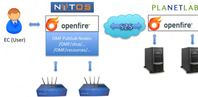
Figure 9: XMPP server to server peering in OMF
