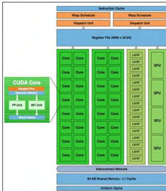
Figure 3.3 – A streaming multiprocessor
