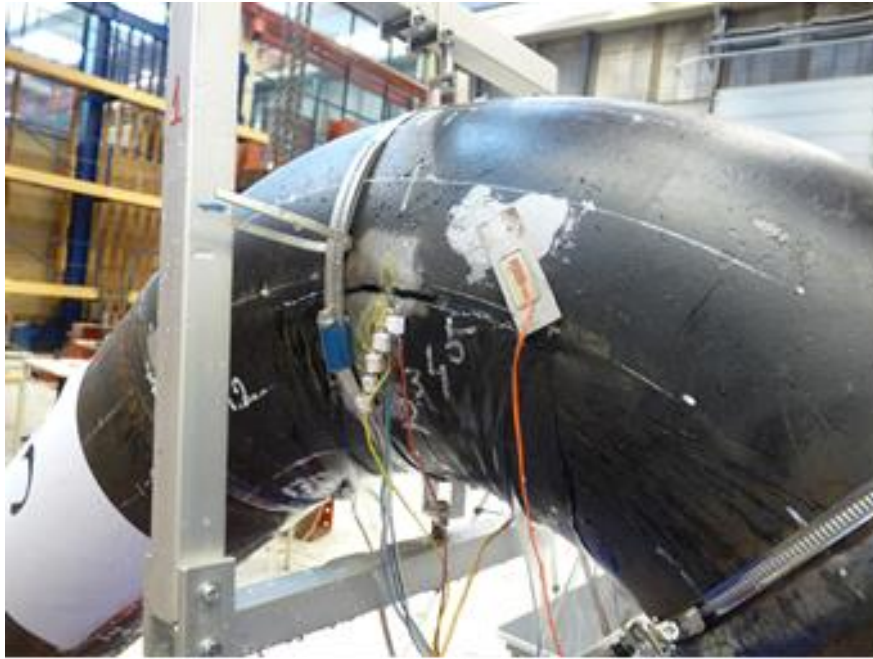
Figure 4. 6: Crack location at the elbow “flank”.
