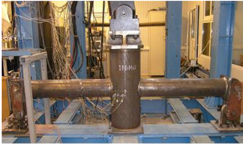
Figure 5.2: Test configuration for IPB loading.
