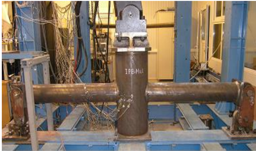
Figure 5.2: Test configuration for IPB loading.
