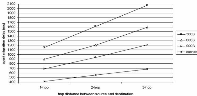
Fig 8.8 Agent migration delay as a function of hop distance for different agent sizes.
