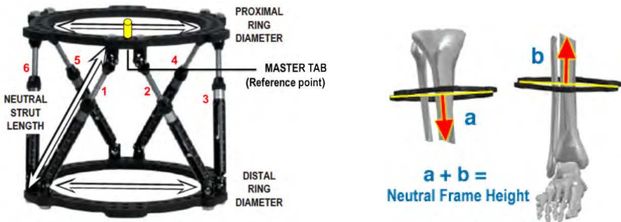
Figure 38: The three parameters that fully describe a configuration are proximal and distal internal diameter and neutral strut length or frame height (C.Taylor, Correction of General Deformity with the Taylor Spatial Frame Fixator™ , 2002)
