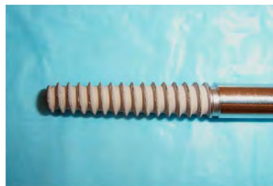
Figure 41: HA is a naturally occurring mineral form of calcium apatite, which makes up to 50% of bone in its inorganic phase. It is commonly used to coat implants (e.g. hip replacements) since it has been suggested that it promotes osseointegration. (Fragomen et al., 2006)
