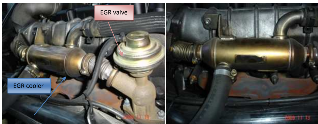
Figure 46 DW10 EGR complete system (left) and EGR cooler details (right)
