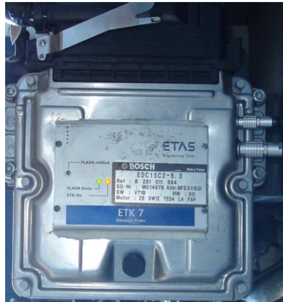
Figure 2 BOSCH EDC 15C2 Engine Control Unit
