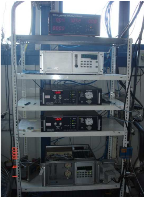
Figure 1 Exhaust gas analyzers
