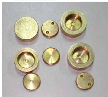
Figure 5.4. Copper build up caps for 6 and 15 MV.
