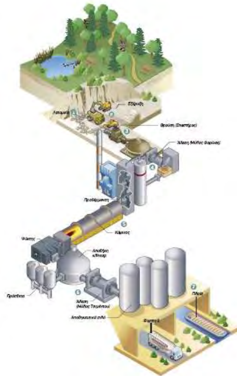
Figure 2.1: Basic flow sheet of cement production
