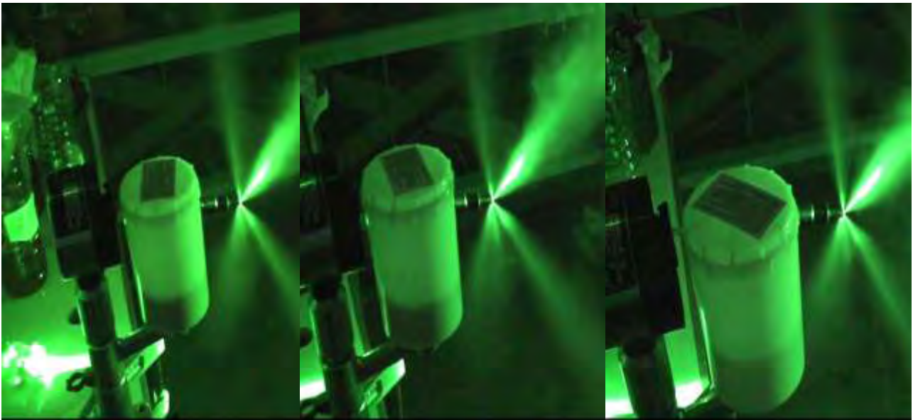
Figure 9.16. Closer view of spray evolution of RF91 injector for B0, B60 and B100 fuels under specific injection conditions. P_{inj} = 210 bar, P_{amb} = 1.01 bar.
