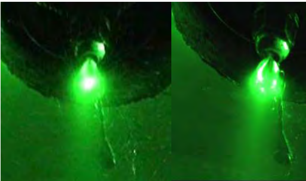
Figure 9.17. Comparison of spray evolution (closer view) using low pressure nozzle for B40 and B100 fuels (1 cm from the tip of the nozzle) under specific injection conditions. P_{inj} = 10 bar, P_{amb} = 1.01 bar.
