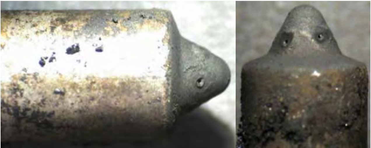
Figure 8.5. 1 st cylinder Common Rail injector magnified view after 30 h operation with B70 fuel.
