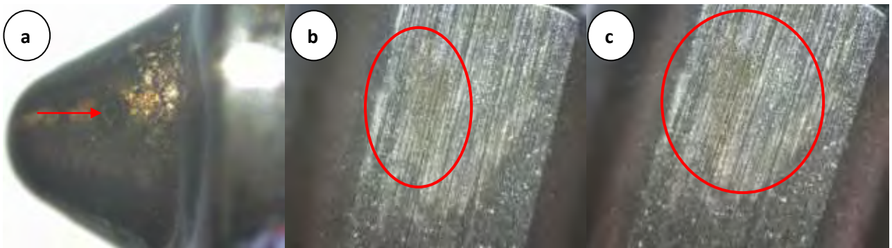
Figure 8.14. After cleaning magnified view of the 2 nd injector nozzle holes (a), and plunger (b) and (c).
