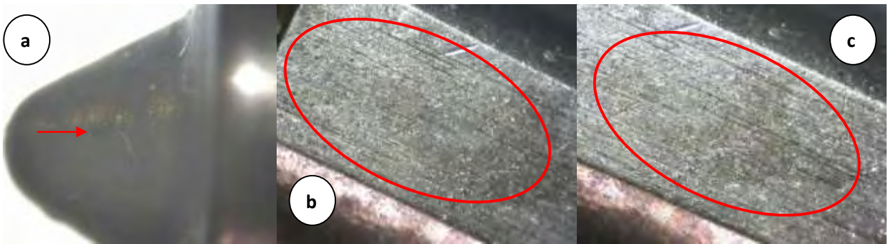
Figure 8.15. After cleaning magnified view of the 3 rd injector nozzle holes (a), and plunger (b) and (c).
