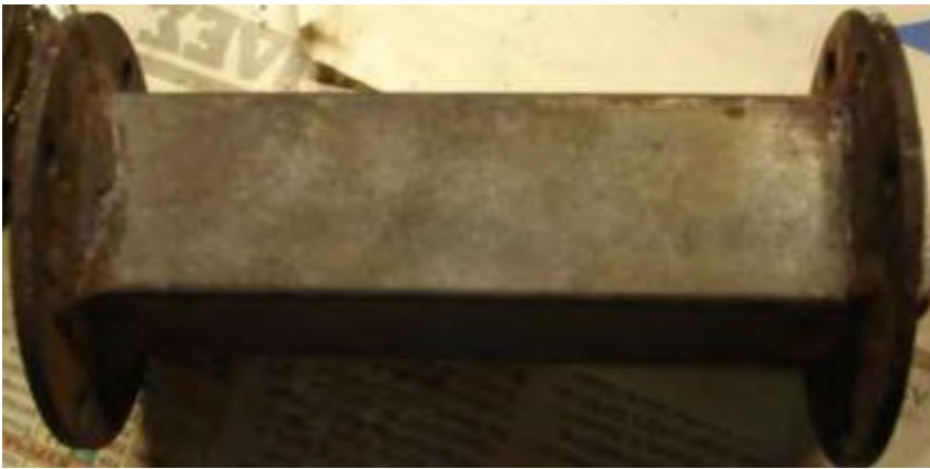
Figure 7.1. SiC filter view, monitored filter's lateral surface.
