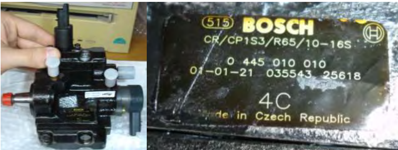
Figure 8.18. Brand new Bosch high pressure pump (left) and model characteristics (right).
