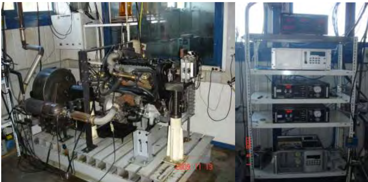
Figure 3.1. DW10ATED engine test bench (left) and group of Exhaust gas analyzers (right). DW10 HDi Diesel engine, eddy current dynamometer and exhaust system are presented.
