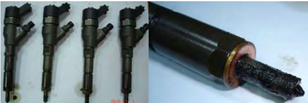
Figure 8.4. Used Common Rail injectors (left) and closer view of the deposits (right).
