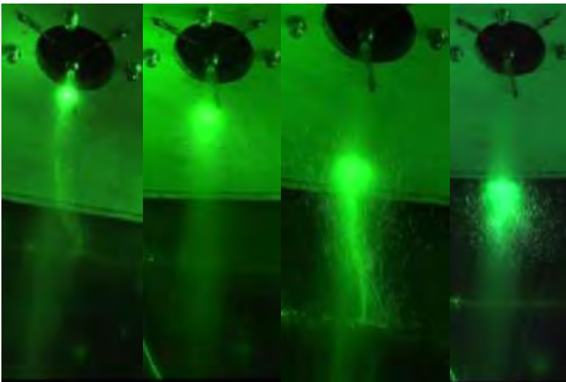
Figure 9.25. Spray evolution using low pressure nozzle for B40 fuel at several positions from the tip of the nozzle and under specific injection conditions. P_{inj} = 10 bar, P_{amb} = 1.01 .
