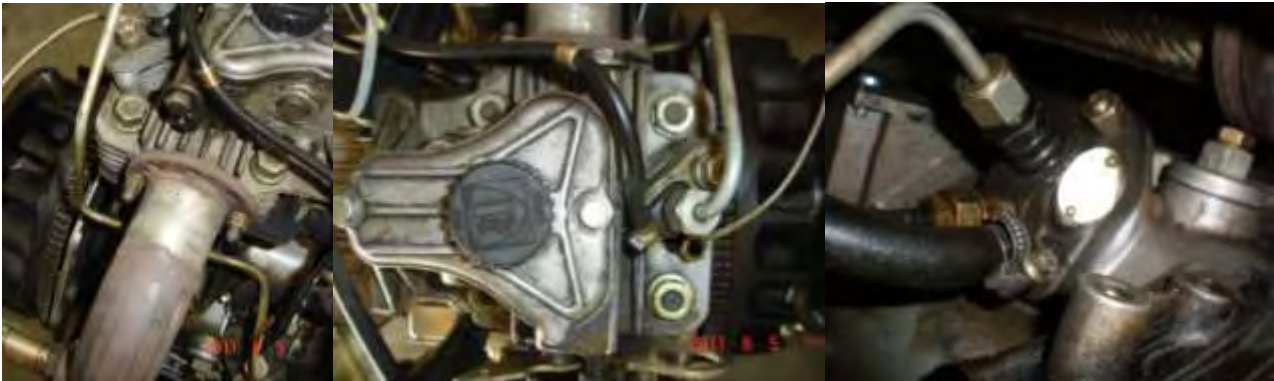
Figure 6.2. High pressure line (left), injector location (centre) and diesel pump (right).
