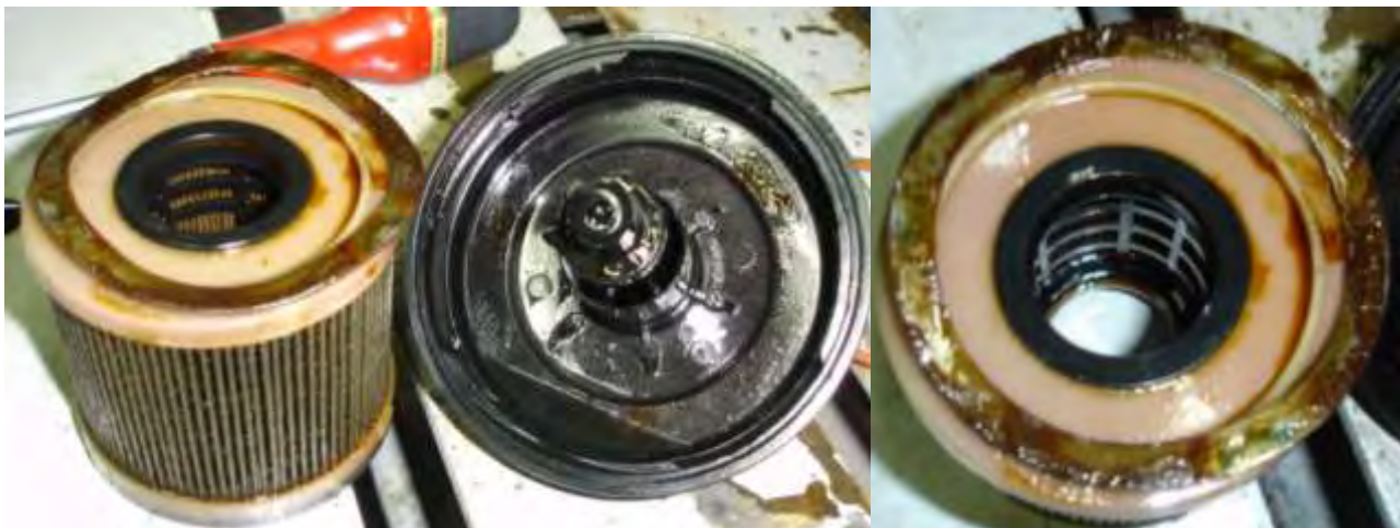
Figure 8.2. Fuel filter condition after 30 h operation with B70 fuel.
