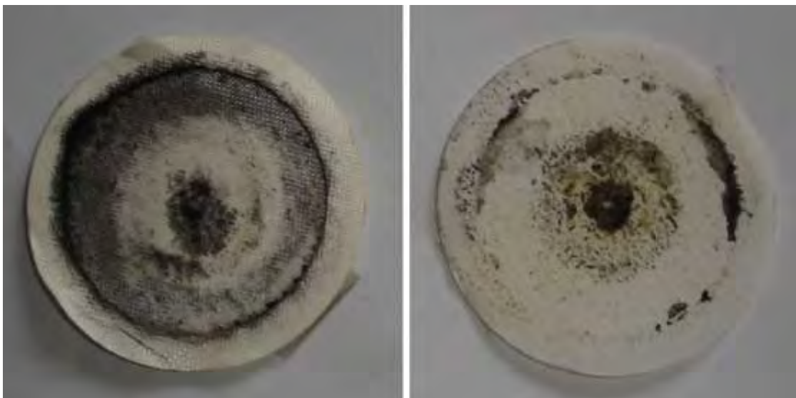
Figure 4.9. Comparison of particulate samples (undiluted exhaust gas upstream filter passing through a Pallflex 47mm filter during the total cycle. Left: Diesel fuel. Right: B70 biodiesel blend.
