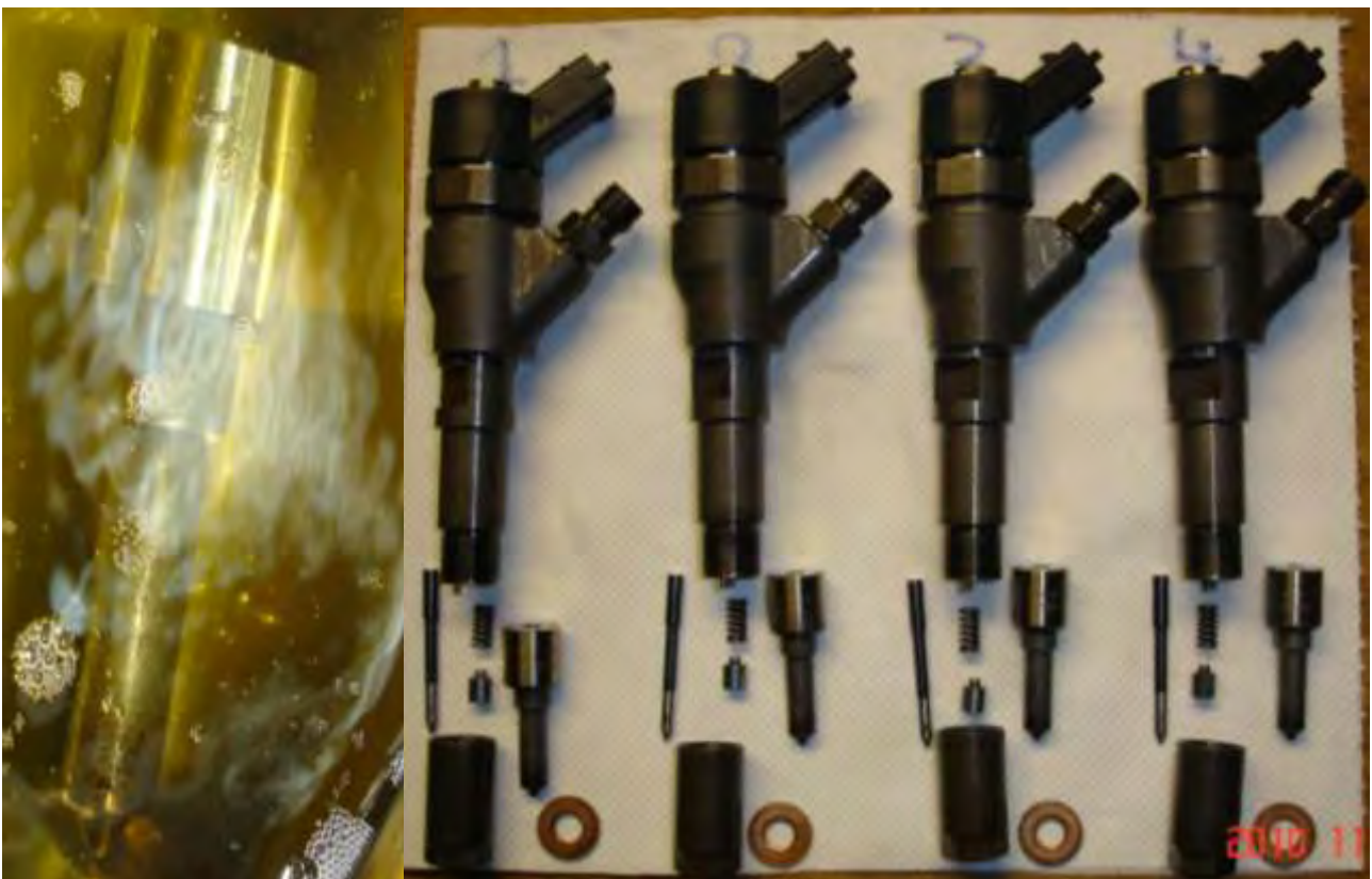
Figure 8.12. Cleaning procedure using ultrasonic bath (left) and disassembly view of the clean injectors (right).
