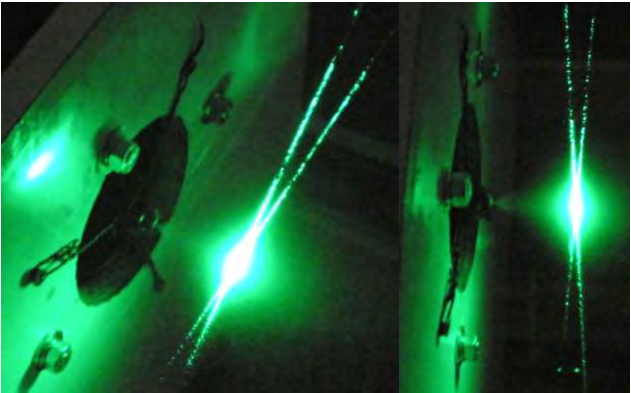
Figure 9.3. Low pressure diesel spray. Green laser beams and cross-section area (measurement volume) are clearly observable.
