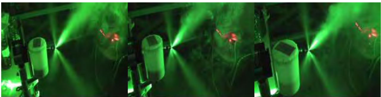
Figure 9.15. Differences in spray evolution of RF91 injector for B0, B60 and B100 fuels under specific injection conditions. P_{inj} = 210 bar, P_{amb} = 1.01 bar.
