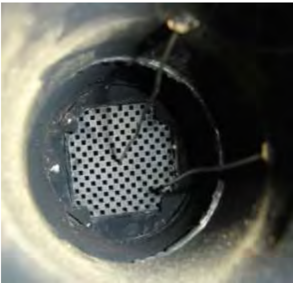
Figure 7.2. Thermocouples positions at the selected filter exit channels.
