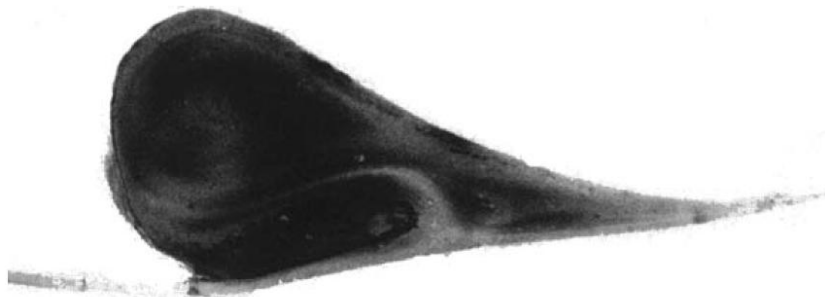
Figure 3.3. Experimental flow pattern in the melt bank of calendered PVC [11, 12].
