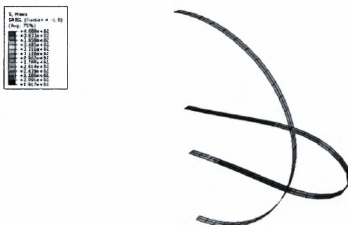
Figure A.1.5. Large deformations due to cross-section ovalization for large value of curvature for the elastic strip using shell elements with S4R302 mesh type
