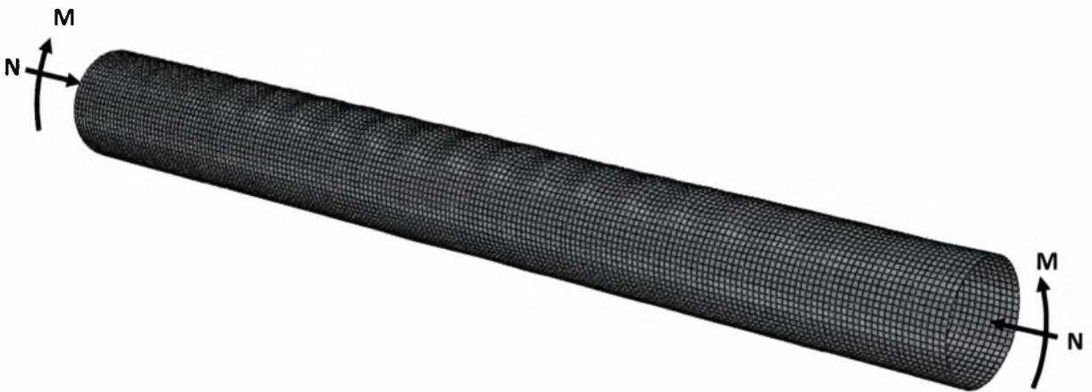
Figure 6.3.1 Loading and model configuration of the imperfect tubular member with D=323.9\text{mm} , t=10\text{mm} and L=3\text{m} ( w_0=0.5t )
