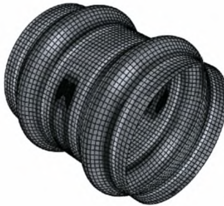
Figure 5.1.1.8 Failure mode for the model with D=355\text{mm} , t=12\text{mm} and L=0.5\text{m} ( \lambda=0.07 ) with e_0=L/500
