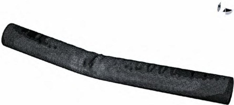
Figure 6.3.3a Deformed geometry of the tube model with D=323.9\text{mm} , t=10\text{mm} and L=3\text{m} ( w_0=0.5t ) under axial compression up to 0.25N_a and bending.
