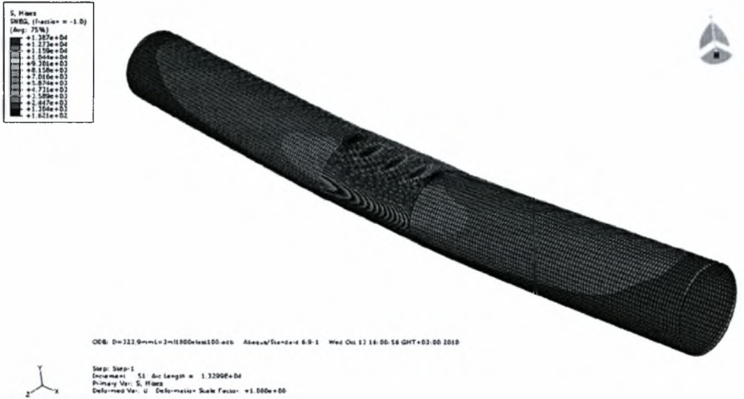
Figure A.2.7 Post buckling behavior where local buckling occurs and wrinkling development for mesh type 2, point 1
