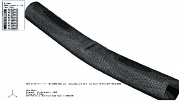
Figure 6.1.7 Deformed tubular member with D=355\text{mm} , t=12\text{mm} , L=3\text{m} and e_0=L/1000 under combined loading with 0.25N_a
