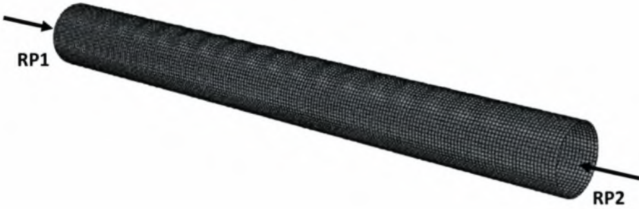
Figure 4.3.1 Simulation of the wrinkled model with w_0/t=0.5 under axial compression
