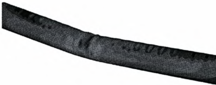
Figure 6.3.6 Failure geometry for the model with D=323.9\text{mm} , t=10\text{mm} , L=3\text{m} with w_0=0.5t and constant axial compression equal to 0.25N_p
