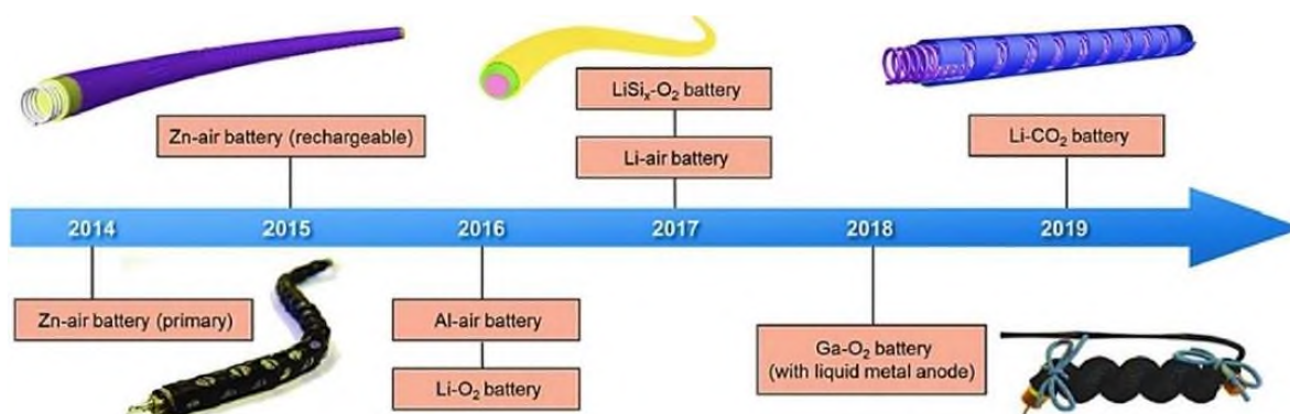
Figure 5.28 Schematic showing the progress made in the development of fiber-shaped metal-air batteries [345, 440].
