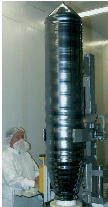
Figure 3.1: Czochralski silicon crystal with a diameter of 300 mm and a weight of more than 250 kg [32]
