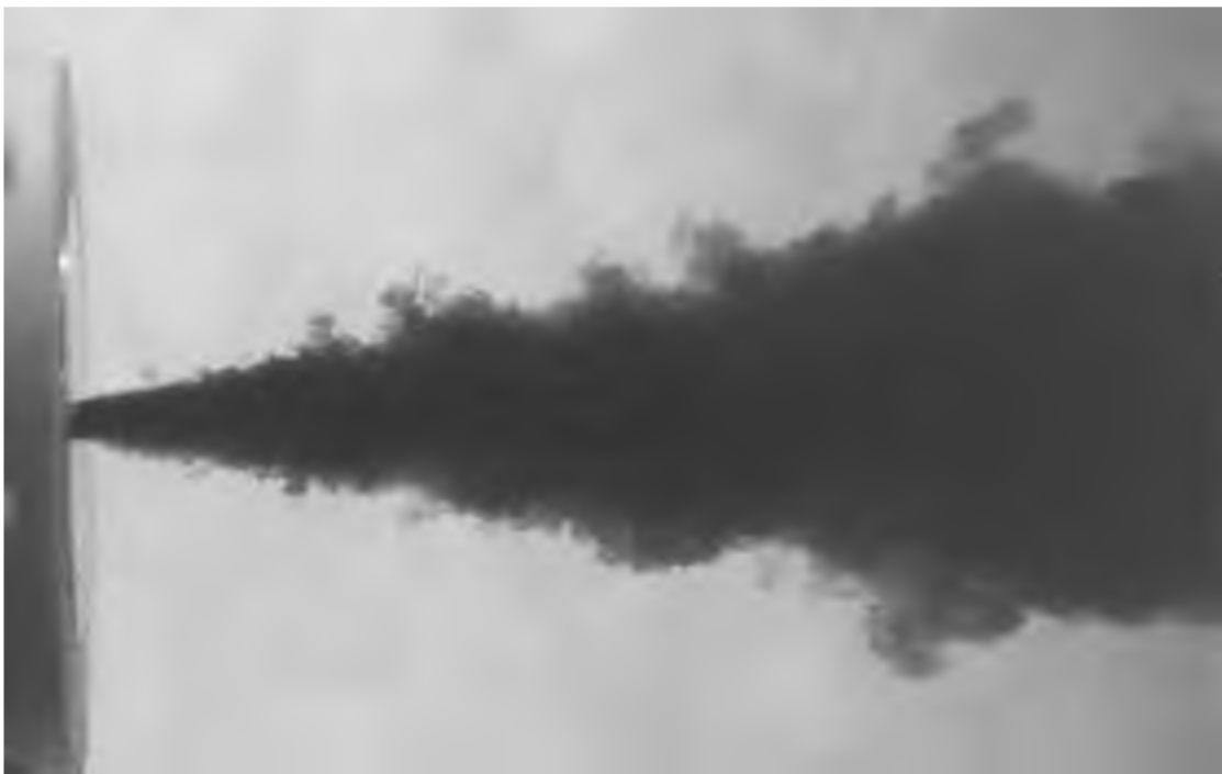
Figure 2-8 A water jet emanating from a nozzle round orifice into an undisturbed tank of water, Benoit Cushman-Roisin [70]
