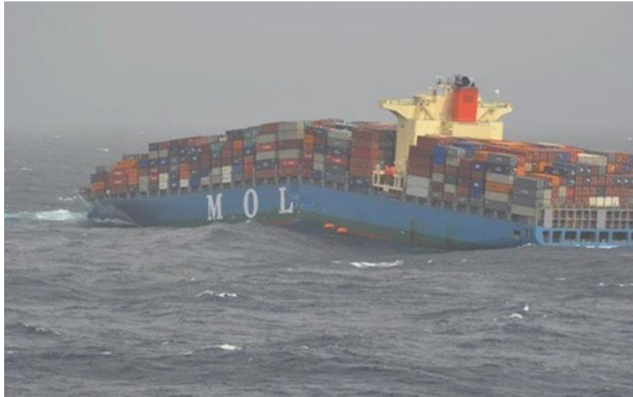
Figure 60: MOL Comfort after the failure of her hull.
