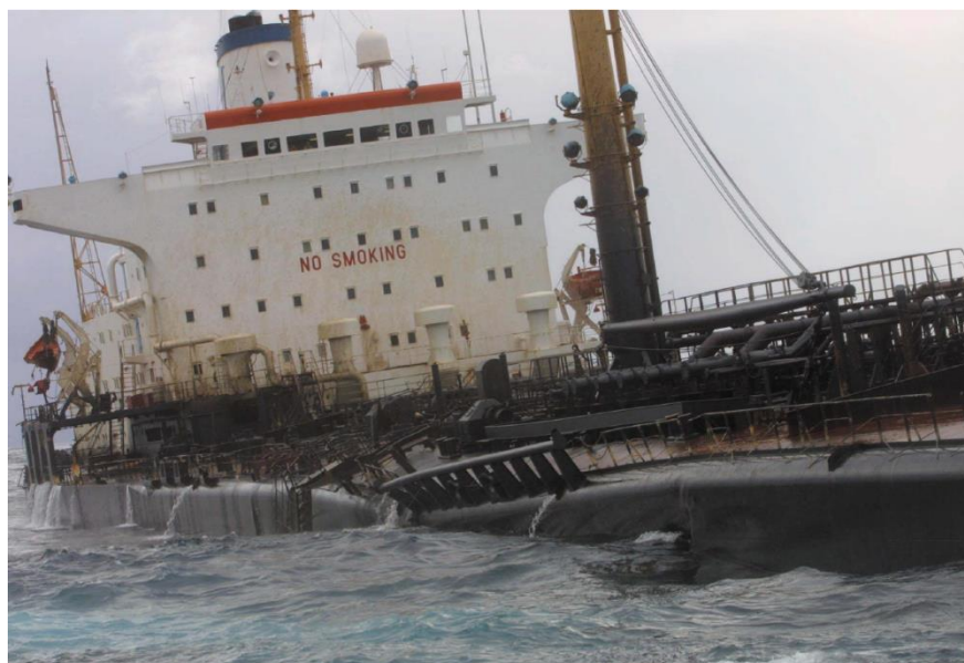
Figure 58: The damage of the starboard side and the preexisting permanent deformations from STS operations at the side shell plating.
