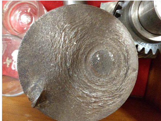
Figure 48: Example of fatigue fracture surface.
