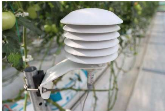
Figure 3.2. Temperature and humidity sensor enclosed in a radiation shield of Thygro SDI-12.
