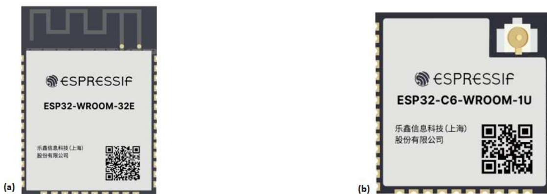
Figure 2.13. (a) ESP-32 WROOM-32E, with Internal antenna, on the left (source: espressif, esp32 documentation) . (b) ESP32-WROOM-32UE, with surface-mount uFL connector for external antennas, on the right (source: espressif, esp32 documentation)
