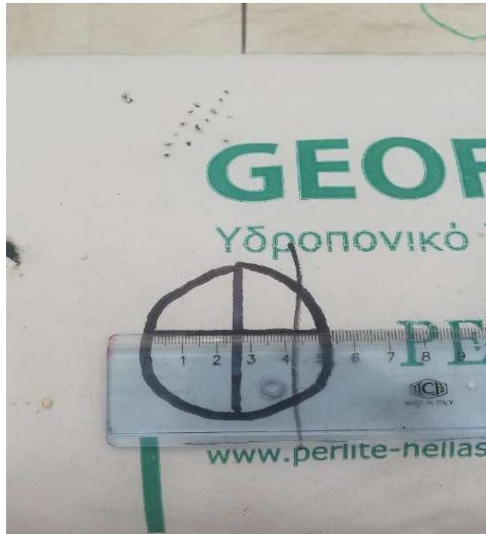
Figure 4.9. A circle of 5 cm diameter was drawn on every slab. Each circle was 10 cm away from the planting area. All the measurements were taken inside the circle to minimize the water content variability.
