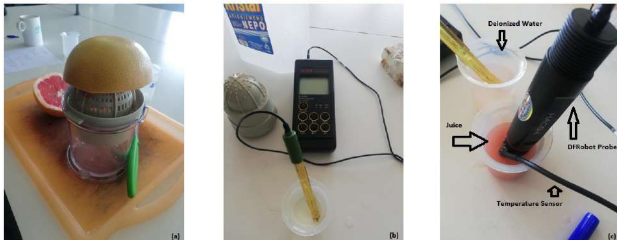
Figure 5.4. (a) The hand squeezing procedure. (b) Hanna pH meter. (c) DFRobot pH meter probe.
