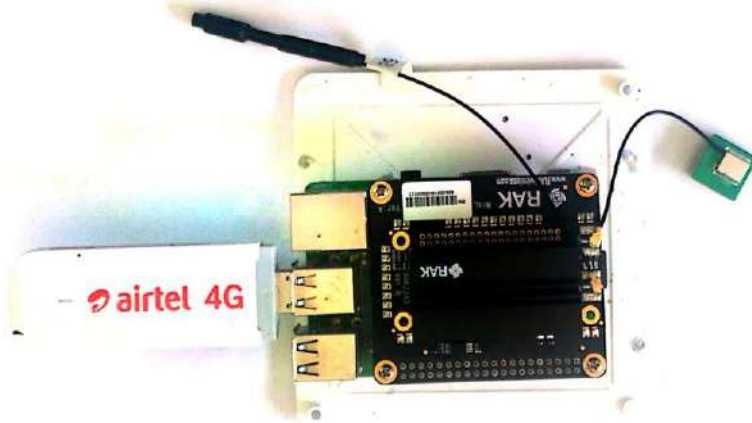
Figure 4.6. Raspberry pi 3 B+ combined with a RAK2245 Pi Hat for LoRa gateway deployment. To connect to the server a 4G/LTE dongle is added with a SIM card.
