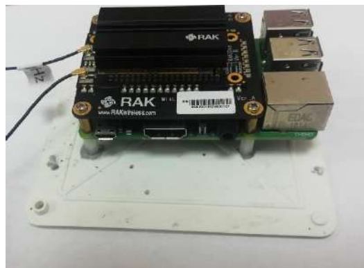
Figure 2.15. Raspberry pi 3, model B stacked with a LoraWan Gateway with RAK2245 Pi Hat. This is the gateway where all the LoRa nodes send their data. The Raspberry Pi connects via WiFi or 4G (dongle) to upload the data to an IOT server in case no internet connection is available.
