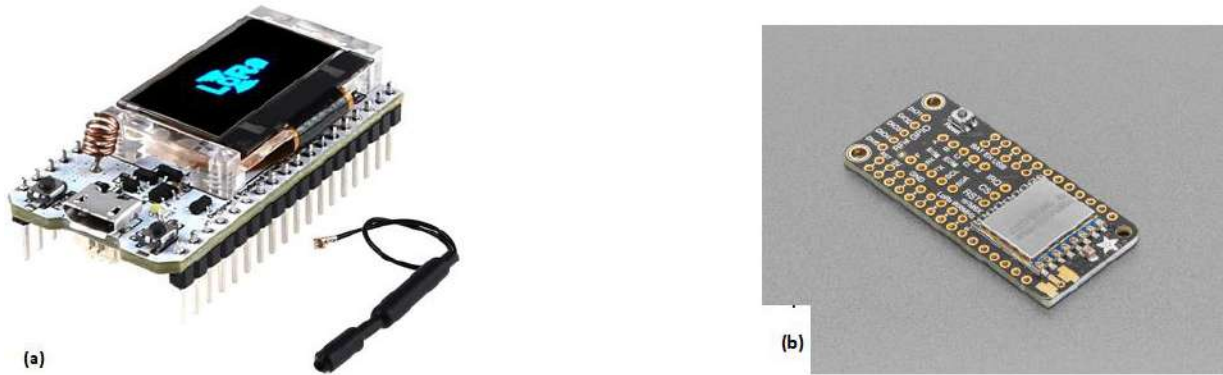
Figure 2.23. (a) OEM LoRa development board embedded with an OLED screen (source: Wirelesslan.gr) (b) Adafruit LoRa radio FeatherWing. A shield for the Adafruit feather development board series (source: Adafruit official web site).
