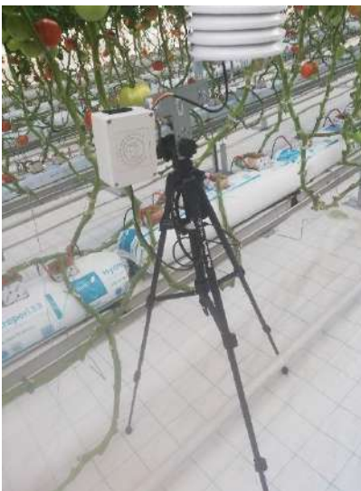
Figure 3.5. The final product for a single system. The box that houses the system is an IP66 plastic box and the body of the station is a camera tripod embedded with aluminum corners that contain mounting holes, which are useful for placing the box in the desirable height.
