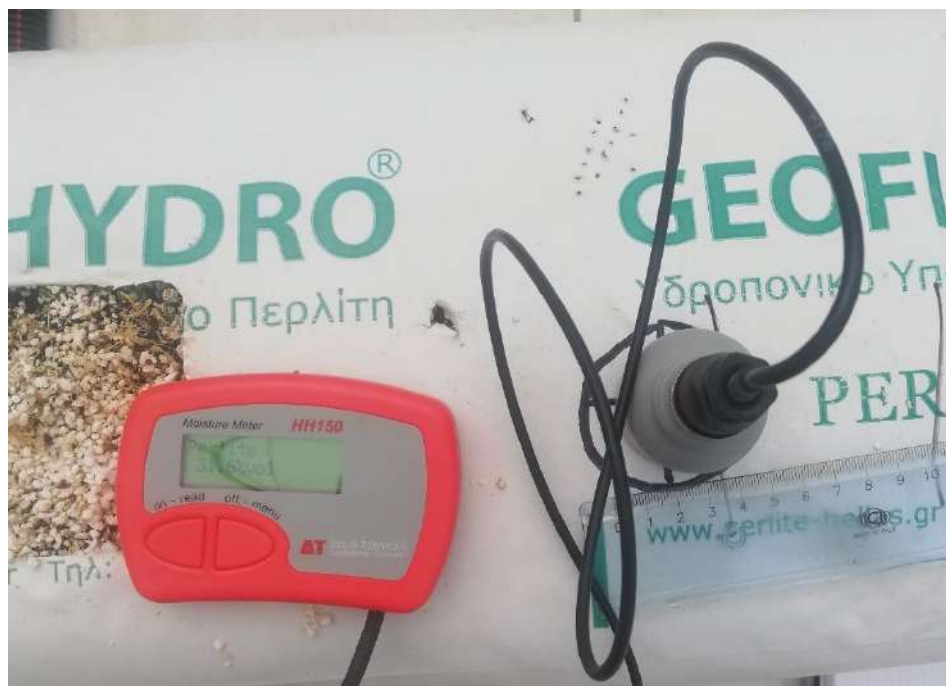
Figure 4.10. HH150 handheld meter and SM150 soil water content sensor. All the measurements are taken with the sensor inserted inside the circle.
