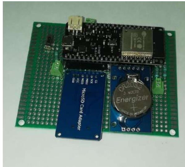
Figure 3.4. Finalized PCB, which does not include the sensor. All the parts were soldered, and the device was tested for 1 week in the lab to make sure everything will work as planned during the field experiment
