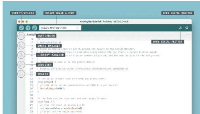
Figure 2.16. Arduino IDE 2. The interface where users can write, compile and upload sketches to the Arduino and Arduino compatible development boards.
