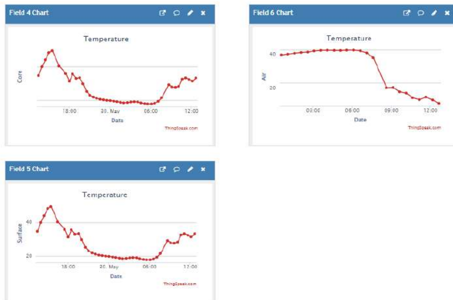
Figure 6.11. ThingSpeak interface. The core, surface and air temperature are visualized using linegraphs. Red dots represent the measurements.
