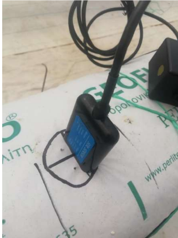
Figure 4.11. Water content sensor connected to the open-source device. The measurement is taken inside the circle, next to the one taken from SM150. Its measurement marks are obvious on the left side of the circle.
