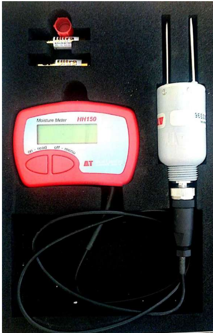
Figure 4.8. HH150 Handheld Meter and SM150 Soil Moisture Sensor used as the industrial device for the method comparison study.
