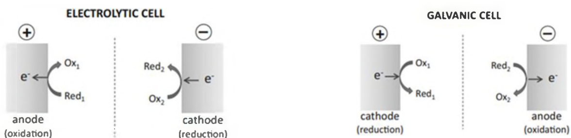
Figure 1. Anode and Cathode in a galvanic an in an electrolytic cell [5]
