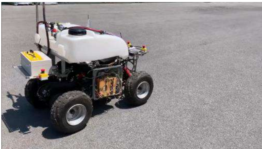
Figure 163: Installation of spraying component at the unmanned vehicle for the needs of iRTA project
