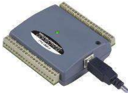
Figure 49: USB-1208LS DAQ device
