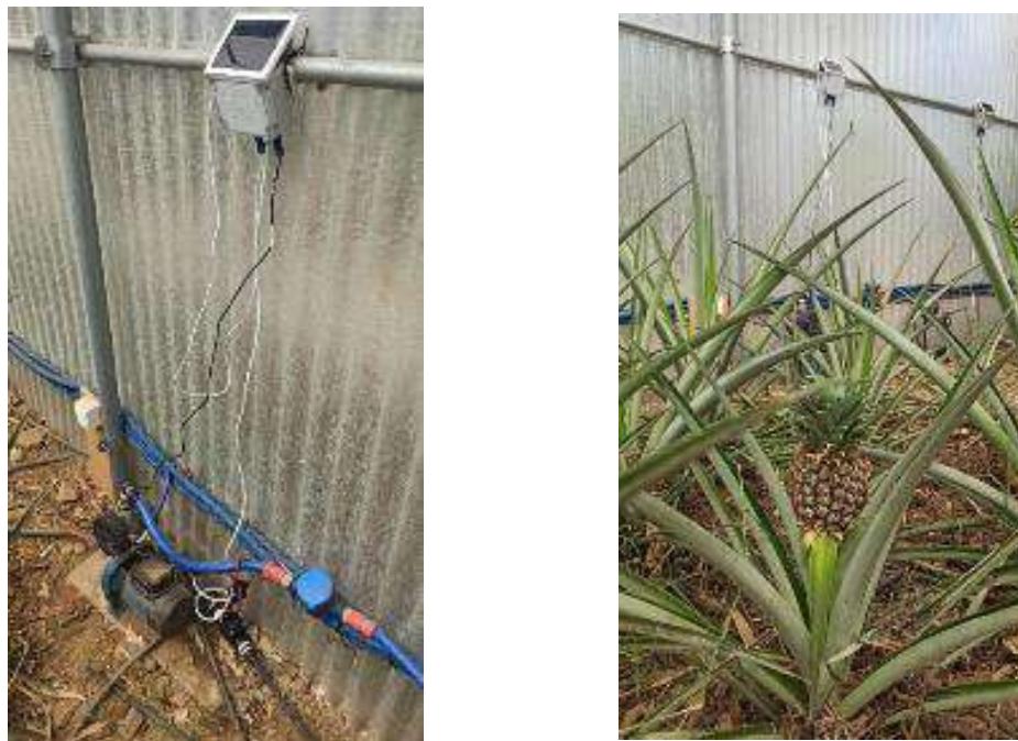
Figure 149: IoT nodes for automating the irrigation in the greenhouse
