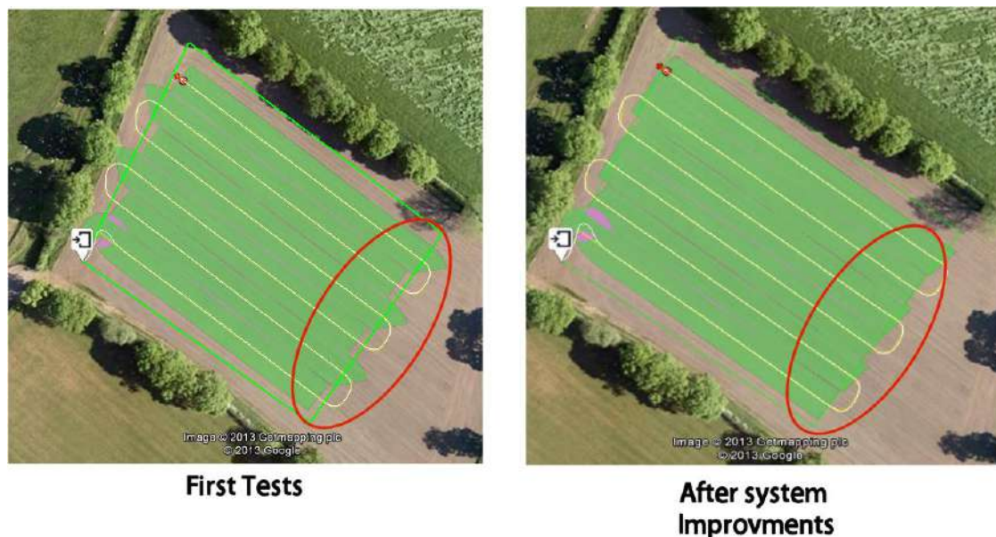
Figure 133: Covered area improvements
