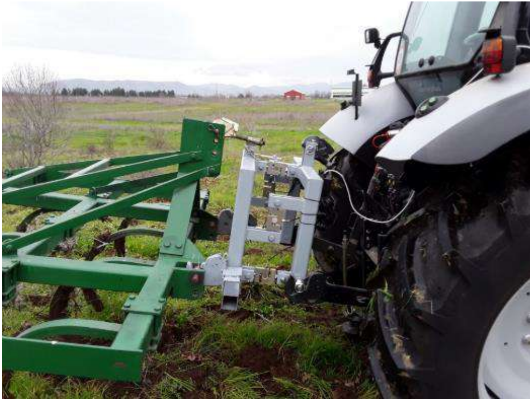
Figure 46: Three-point hitch dynamometer attached to the tractor
