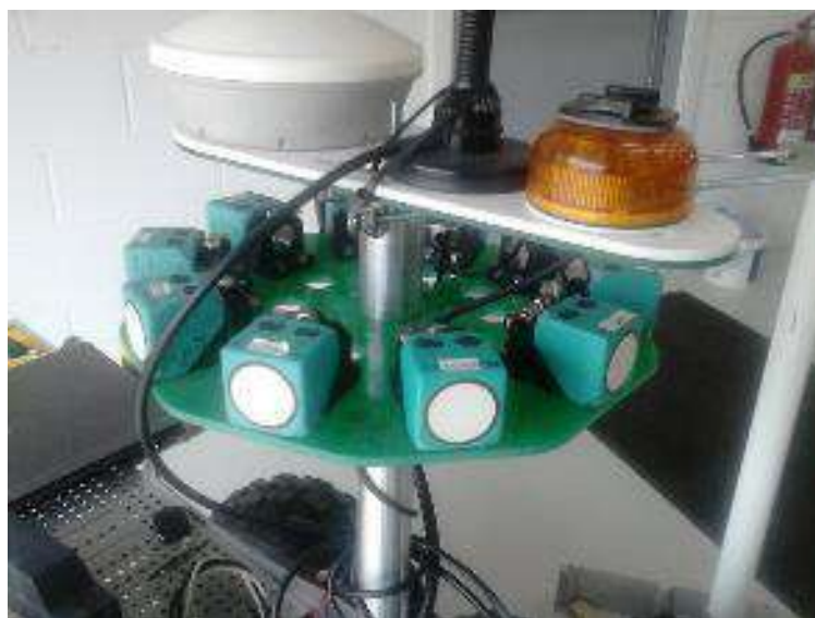
Figure 94: Ultrasonic system with 10 sensors
