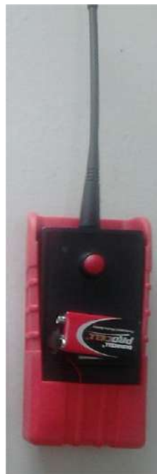
Figure 96: Radio transmitting “dead’s man handle”
