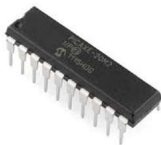
Figure 88: 20M2 PICAXE pic microcontroller chip
