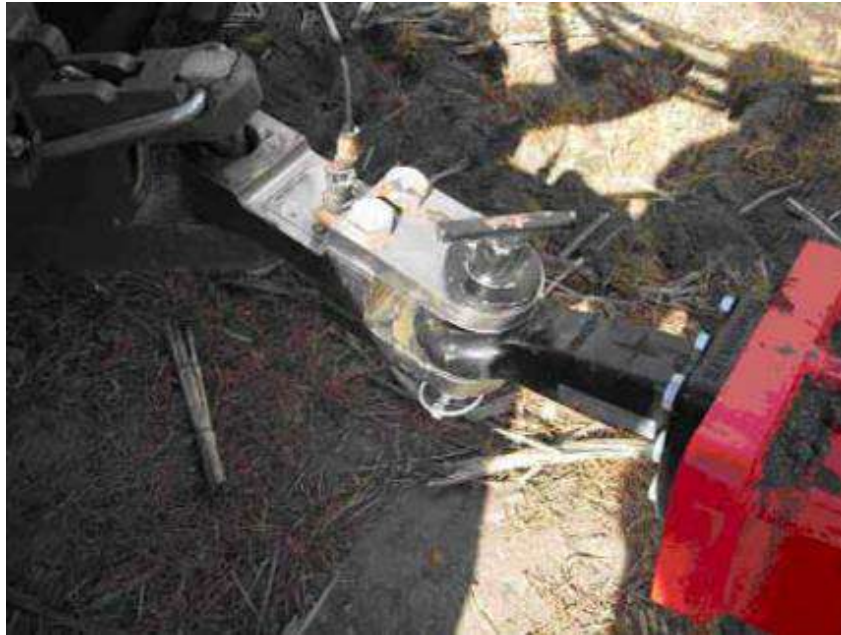
Figure 47: Drawbar dynamometer attached to the tractor
